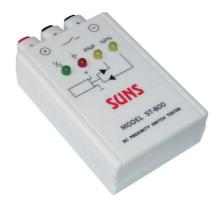
SUNS ST-800 proximity switch tester is designed to test most 3 wire DC proximity switches: inductives [metal sensing], capacitives, photoelectrics or ultrasonics. The unit is fitted with 2x 9V batteries ready for use.
